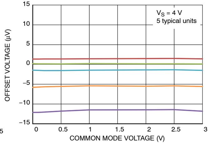
Figure 4. Offset Voltage vs. Common Mode Voltage
