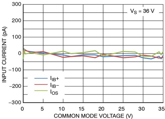
Figure 9. Input Current vs. Common Mode Voltage
