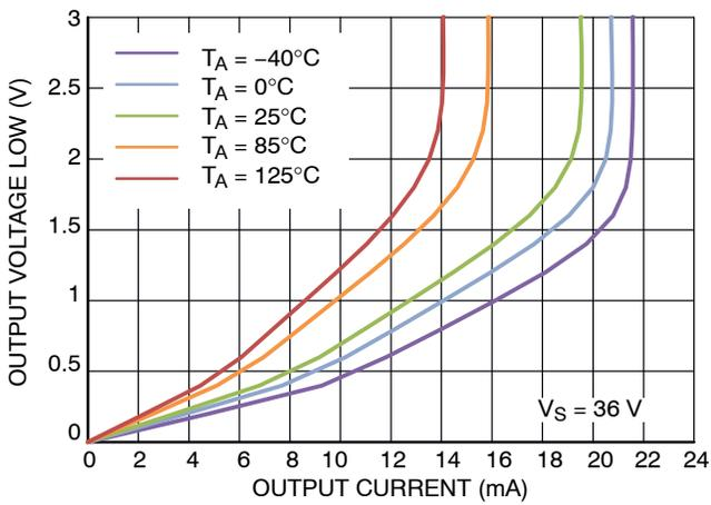
Figure 37. Output Voltage Low vs. Output Current
