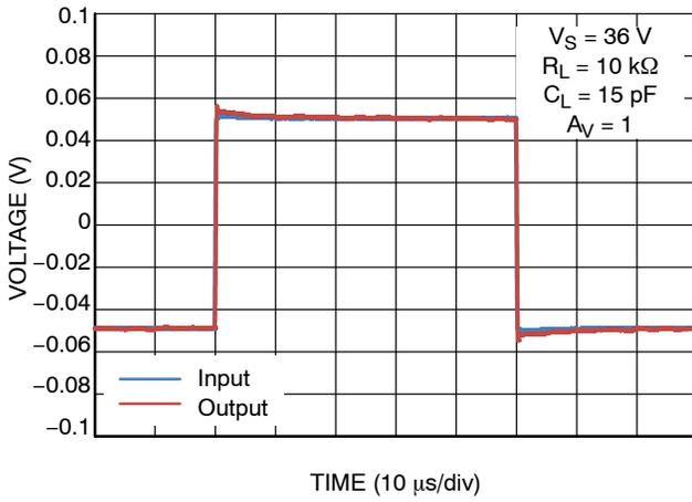
Figure 29. Non-Inverting Small Signal Step Response
