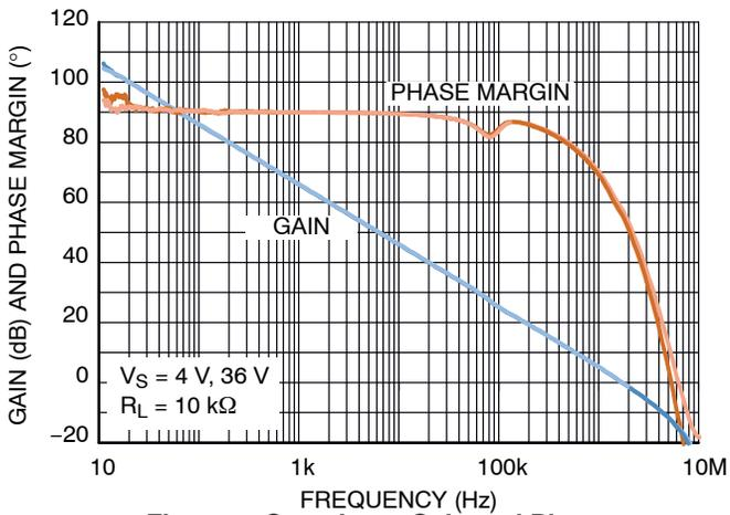
Figure 7. Open Loop Gain and Phase vs. Frequency
