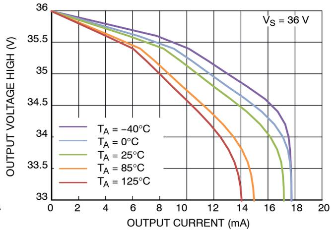
Figure 38. Output Voltage High vs. Output Current
