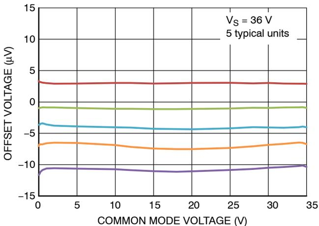
Figure 5. Offset Voltage vs. Common Mode Voltage
