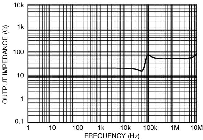
Figure 23. Open Loop Output Impedance vs. Frequency
