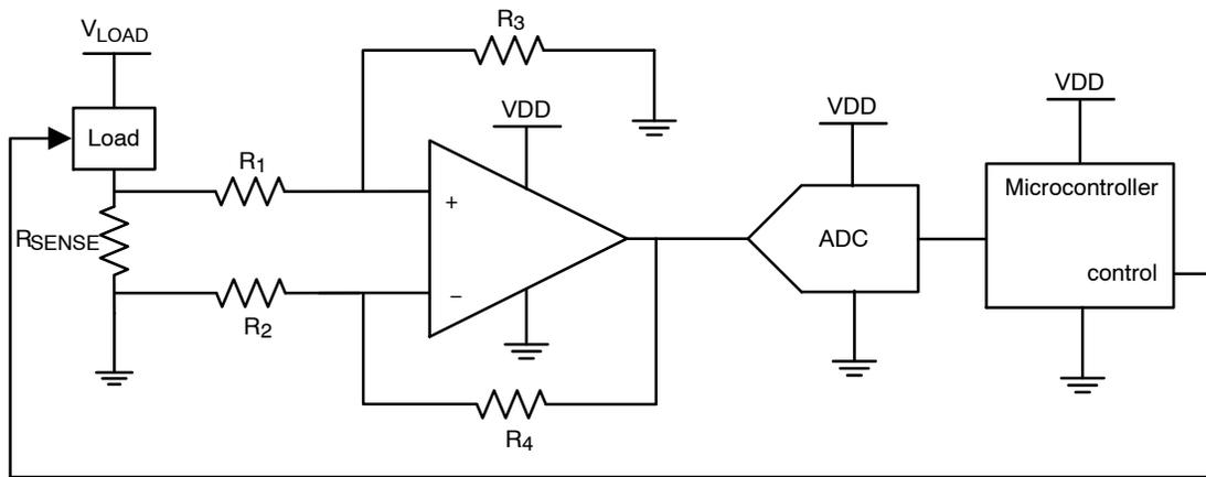
Figure 41. Low-Side Current Sensing
