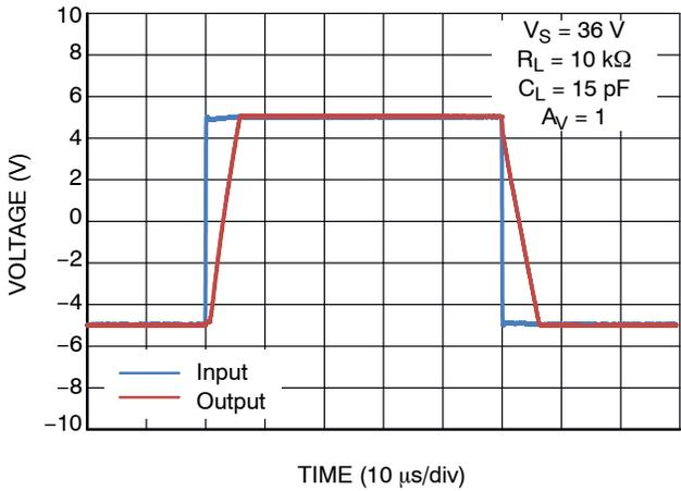
Figure 31. Non-Inverting Large Signal Step Response
