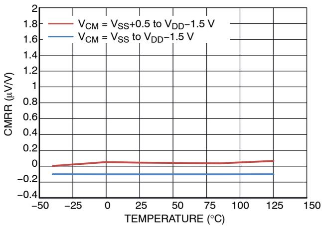
Figure 15. CMRR vs. Temperature at  $V_S = 36\text{ V}$
