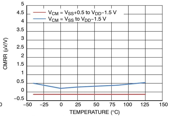
Figure 14. CMRR vs. Temperature at  $V_S = 4\text{ V}$
