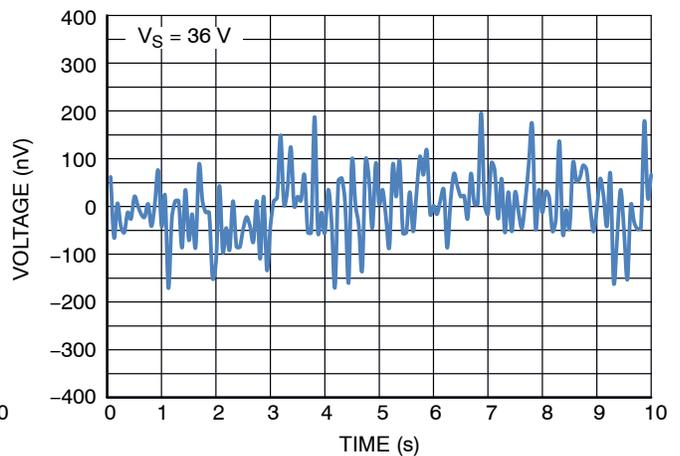
Figure 16. 0.1 Hz to 10 Hz Noise
