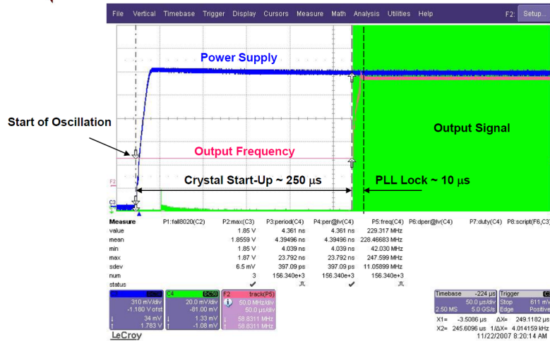
Figure 16. Crystal Oscillator Start-Up vs PLL Lock Time
