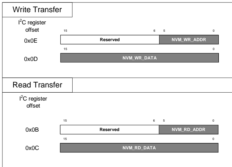
Figure 31. EEPROM Direct Access Using I 2 C
