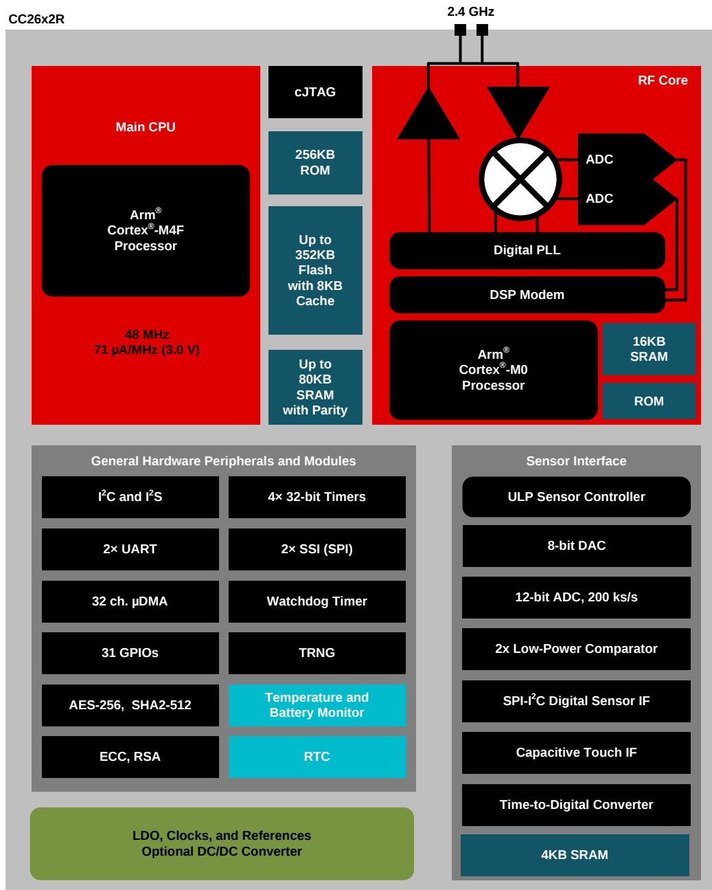
Figure 1-1. CC2642R Block Diagram
