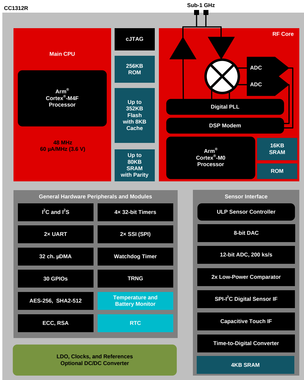
Figure 1-1. CC1312R Block Diagram
