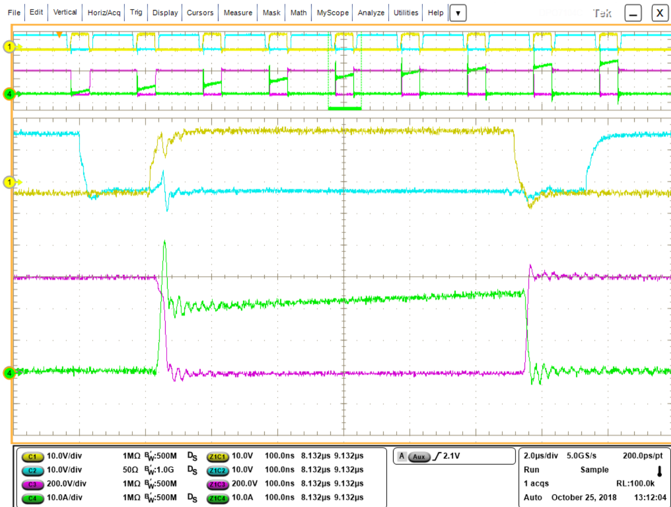
图 43. SiC MOSFET Switching Waveforms
