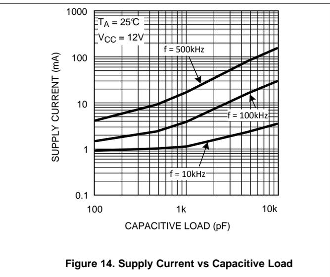
Figure 14. Supply Current vs Capacitive Load
