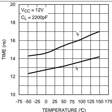
Figure 6. Rise and Fall Time vs Temperature
