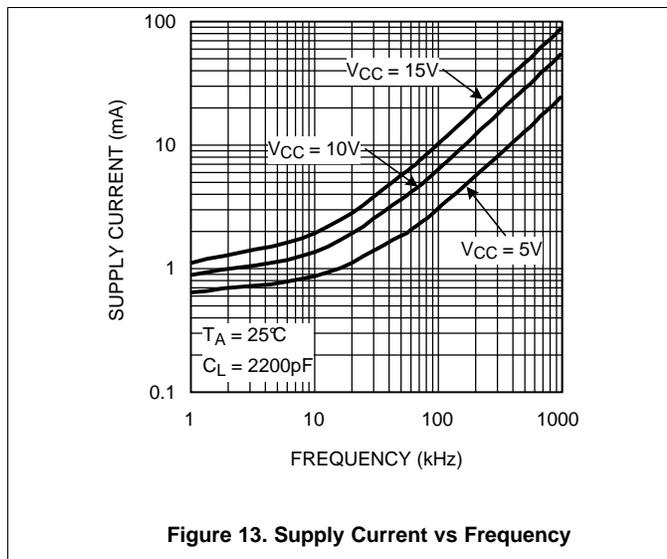
Figure 13. Supply Current vs Frequency
