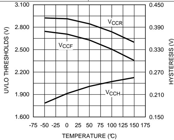
**Figure 11. UVLO Thresholds and Hysteresis vs Temperature**
