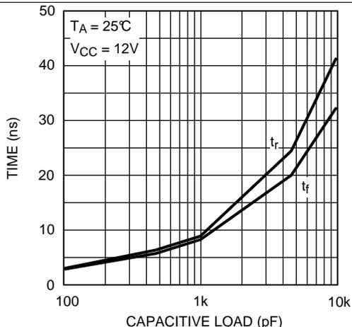
Figure 7. Rise and Fall Time vs Capacitive Load
