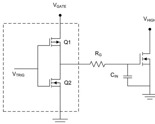
**Figure 16. Driver Output Stage and Load**
