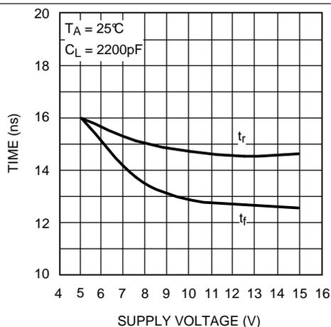
Figure 5. Rise and Fall Time vs Supply Voltage
