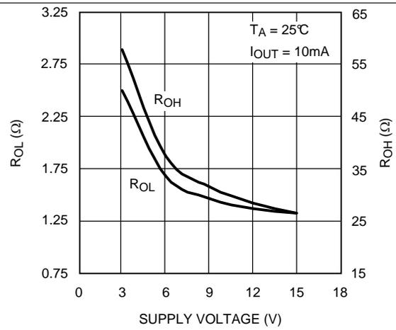
**Figure 10. R<sub>DS(on)</sub> vs Supply Voltage**
