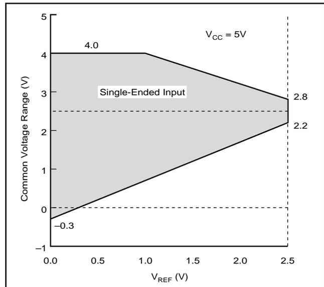
FIGURE 2. Single-Ended Input: Common Voltage Range vs  $V_{REF}$ .
