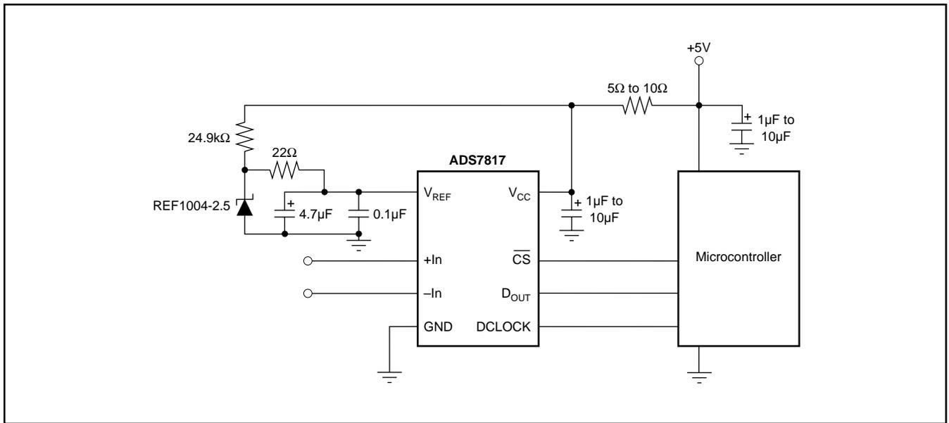
FIGURE 9. Low Cost, Low Power Data Acquisition System.
