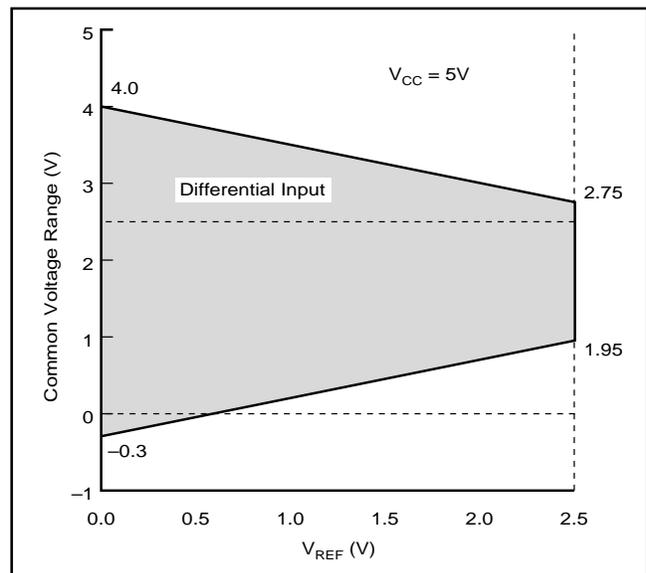
FIGURE 3. Differential Input: Common Voltage Range vs  $V_{REF}$ .
