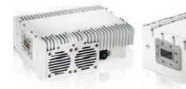
This small and lightweight BUC is ideal for mobile and satellite uplink applications. Designed to be mounted on the feed horn, the BUC has excellent efficiency and consumes less than 250W for 50W C-Band BUC. The unit works on a wide range DC power supply of 38V to 60V. The BUC is able to work up to 60°C. Innovative and efficient thermal design makes this BUC one of the smallest, lightest and most reliable in the industry.
