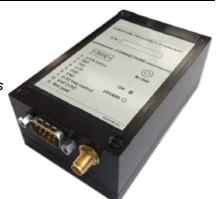
RMRO-10M-Sf-LN-c5 Low Noise Rubidium Oscillator Module is a sub miniature atomic clock combined with 'active noise filter' technology. This rubidium oscillator has 100x less drift than OCXO's. With short term stability of 2x10<sup>-12</sup>/s @ 100s this rubidium oscillator provides significant improvement in performance over other rubidium components
