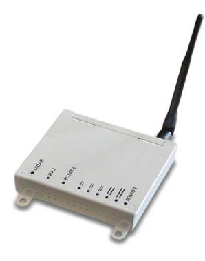
The RWiMAX-3.5-ISU-P2MP-j8 is a 3.5GHz Indoor Subscriber Unit based on our family of low cost subscriber units based on the IEEE802.16-2004 standard.
