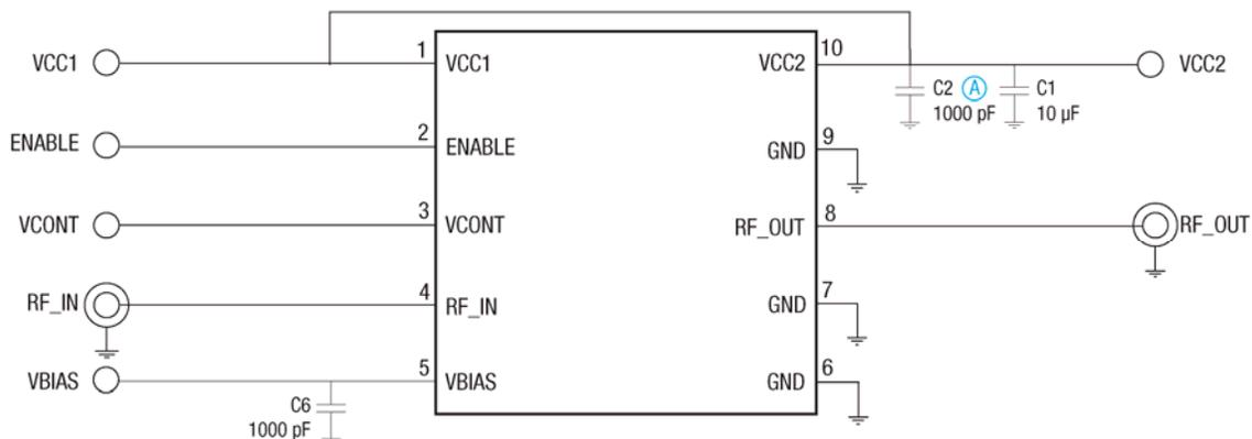
**A** Place caps at closest proximity to PA module with the capacitor grounds directly connected to the PAM grounds. All VCC pins may be connected together at the supply.
