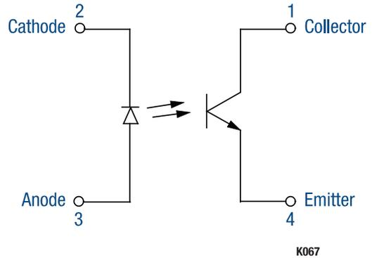
**Figure 1. OLS010 Block Diagram**
