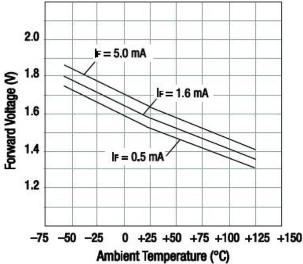
Figure 2. LED Forward Voltage vs Temperature
