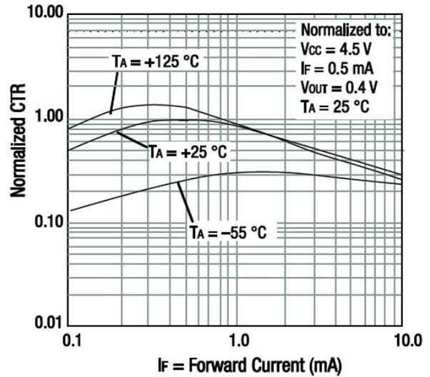
Figure 3. Normalized CTR vs Input Diode Forward Current
