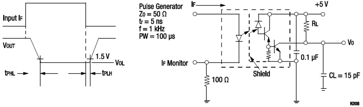
Figure 6. OLH400 Switching Test Circuit
