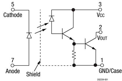
Figure 1. OLH400 Block Diagram
