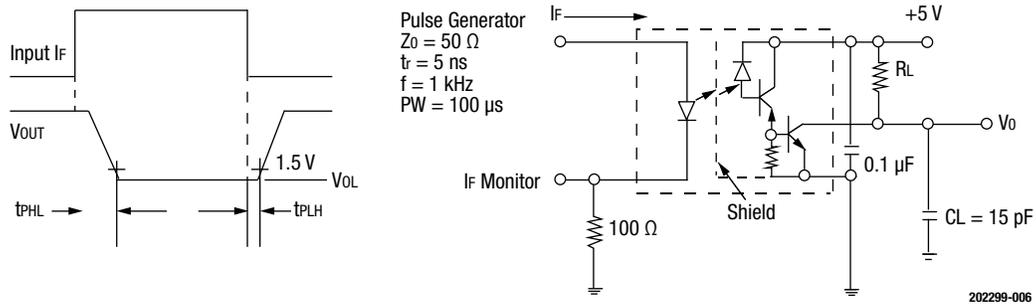
Figure 6. OLH5700/5701 Switching Test Circuit
