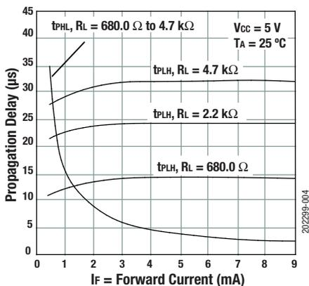
Figure 4. Propagation Delay vs Input Diode Forward Current
