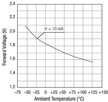
Figure 2. Input Diode Forward Voltage vs Temperature
