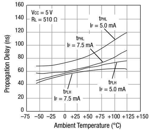
Figure 5. Propagation Delay vs Temperature
