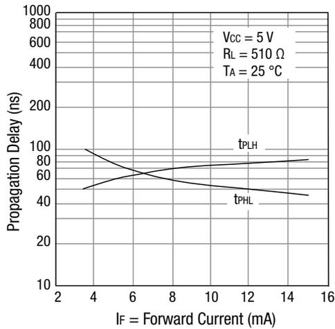
Figure 4. Propagation Delay vs Input Forward Current
