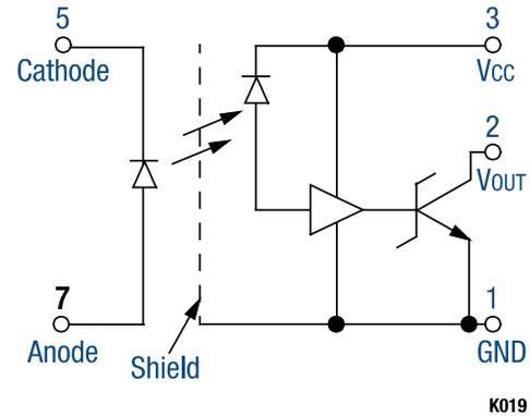
Figure 1. OLH500 Block Diagram
