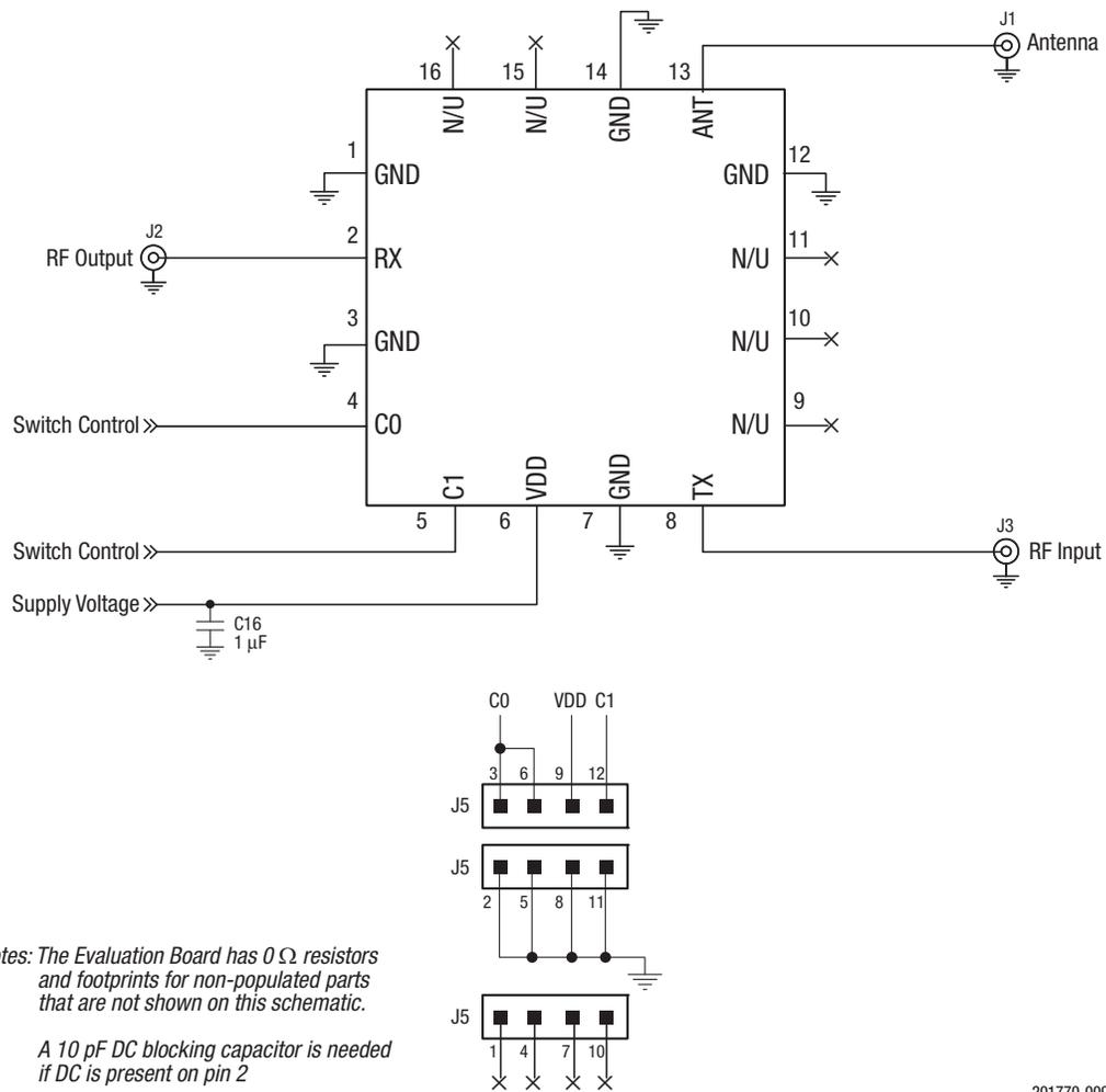
Figure 9. SKY85601-11 Evaluation Board Schematic
