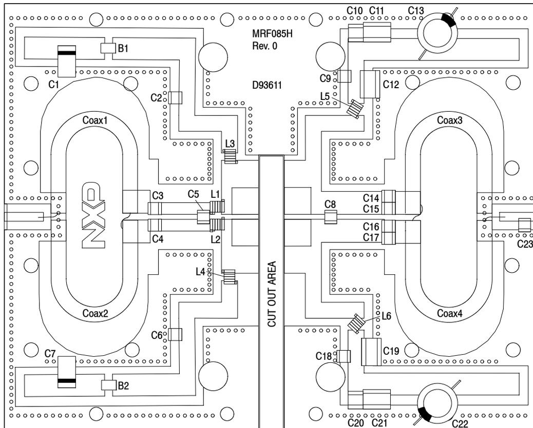
Figure 5. MRF085H Narrowband Test Circuit Component Layout – 520 MHz
