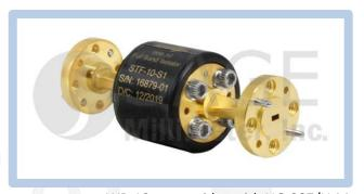
return loss of the isolator is 15 dB. The input and output ports are WR-10 waveguides with UG-387/U-M flanges.
