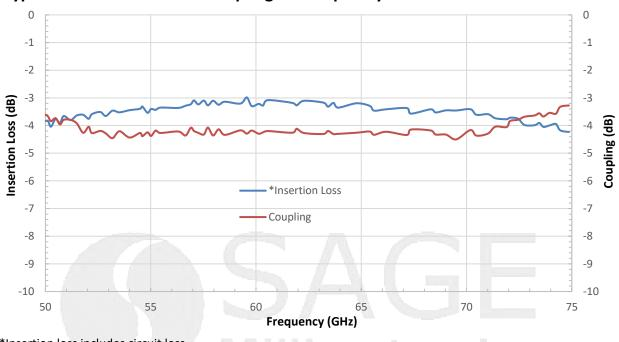
\*Insertion loss includes circuit loss
