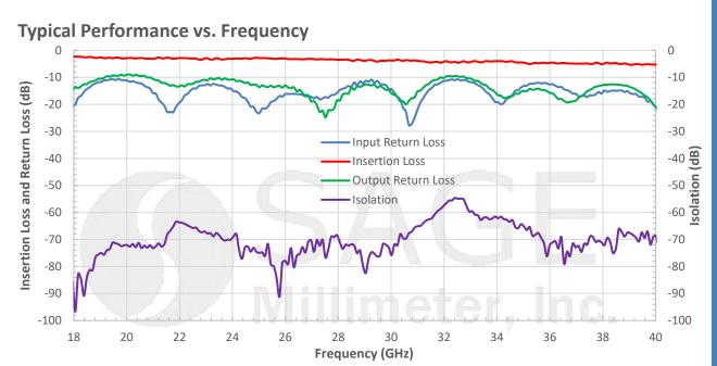
Note: The insertion loss, isolation and return loss between of other ports are similar to the above plot.
