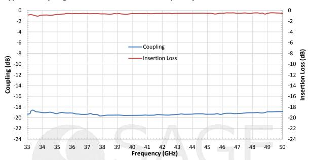
\*Insertion loss includes circuit loss
