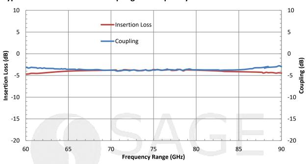
\*Insertion loss includes circuit loss
