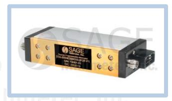
75 dB. The attenuation step sizes are 5 dB. The actuator control and interface circuits are custom designed and uniquely packaged within the attenuator housing. The microprocessor-based electronics ramp the speed of a precision actuator to ensure fast and accurate positioning. The RF connectors are 2.4 mm female. Other connector options are offered under different model numbers. A 9" female to female cable with 10 pin connectors is included for interface convenience.
