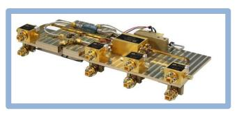
four I/Q mixers for the receivers. The transceiver also includes eight rectangular horns with 10 dB typical gain. The transmitting power of the transmitters is +2 dBm typical for each channel and the conversion loss of the receivers is 12 dB typically. The transceiver assembly requires a typical +6  $V_{DC}$ / 2.3 A DC bias.
