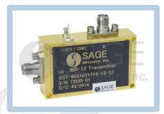
the frequency range of 11.8 to 14.4 GHz. The LO and IF ports are both equipped with female SMA connectors and the RF port has a WR-12 waveguide with a UG-387/U flange.
