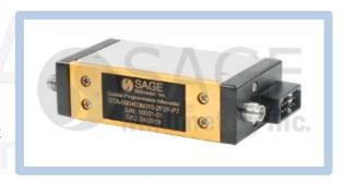
sizes are 5 dB. The actuator control and interface circuits are custom designed and uniquely packaged within the attenuator housing. The microprocessor-based electronics ramp the speed of a precision actuator to ensure fast and accurate positioning. The RF connectors are 3.5 mm female. Other connector options are offered under different model numbers. A 9" female to female cable with 10 pin connectors is included for interface convenience.
