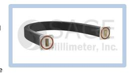
long-term stress free when it is integrated into systems. The flanges of the waveguide are grooved to accept rubber rings to be watertight for outdoor applications. The waveguide is manufactured with a precision manufacturing process to ensure high quality. The waveguide has low insertion loss in the frequency range of 7.05 to 10 GHz. Additional standard lengths and custom length options are available under different model numbers.
