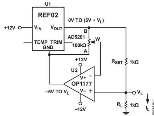
Figure 40. Programmable 0 mA to 5 mA Current Source
