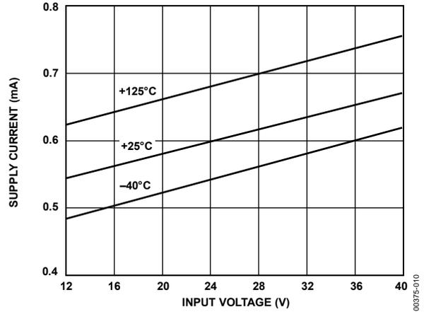
Figure 10. REF01 Supply Current vs. Input Voltage
