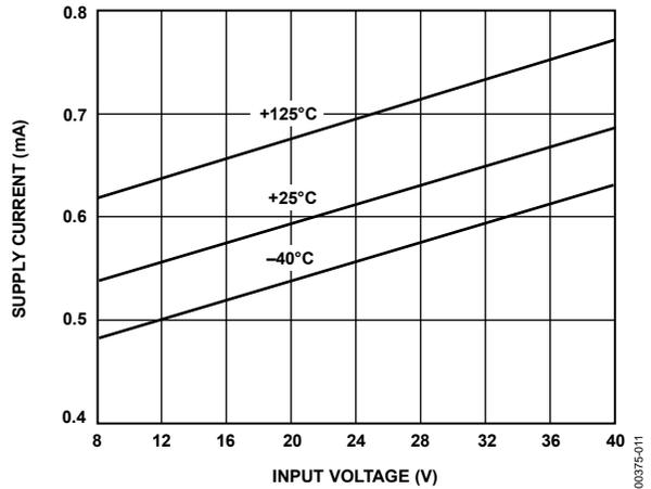
Figure 11. REF02 Supply Current vs. Input Voltage
