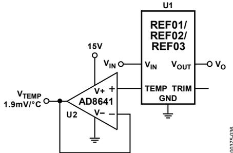
Figure 36. Temperature Monitoring
