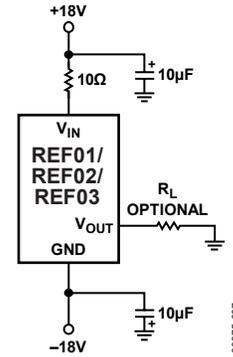
Figure 37. Burn-In Circuit
