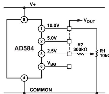
Figure 4. Output Trimming
