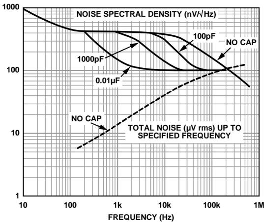
Figure 10. Spectral Noise Density and Total RMS Noise vs. Frequency
