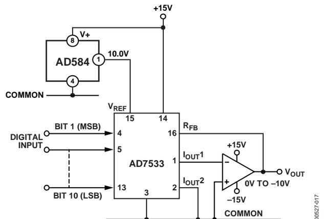
Figure 16. Low Power 10-Bit CMOS DAC Application
