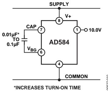
Figure 9. Additional Noise Filtering with an External Capacitor
