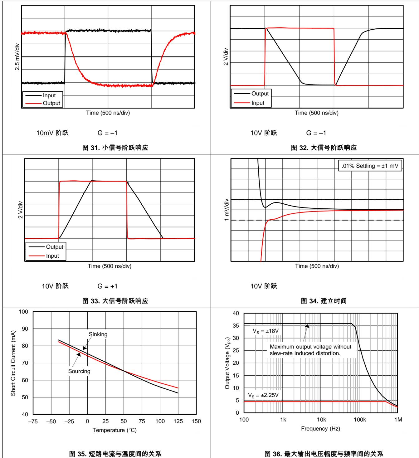
$T_A = 25^\circ\text{C}$  时,  $V_S = \pm 18\text{V}$ ,  $V_{CM} = V_S / 2$ ,  $R_{LOAD} = 10\text{k}\Omega$  已连接至  $V_S / 2$ , 并且  $C_L = 100\text{pF}$  (除非另有说明)
