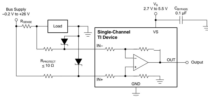
图 49. Transient Protection Using Dual Zener Diodes
