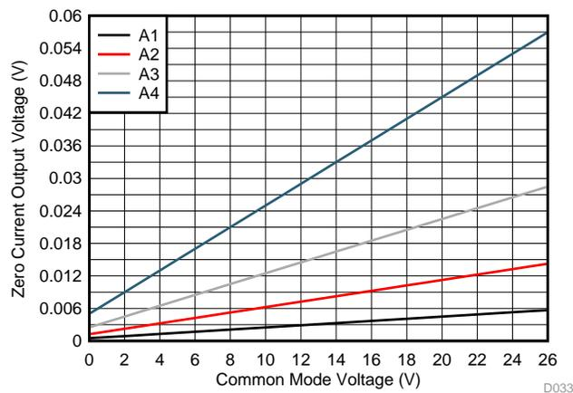
**图 43. Zero-Current Output Voltage vs Common-Mode Voltage**
