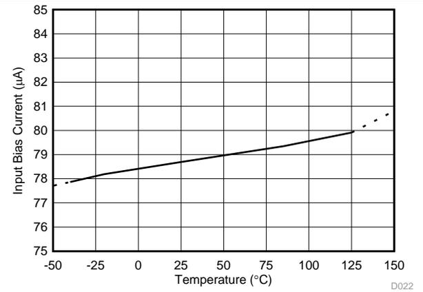
图 22. Input Bias Current vs Temperature
