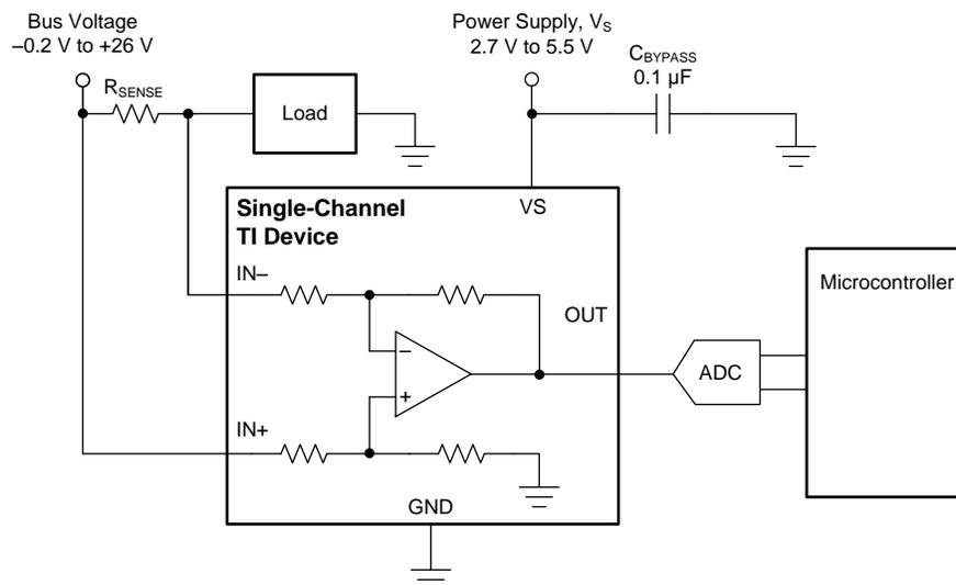
NOTE: For best measurement accuracy, connect analog-to-digital converter (ADC) reference or microcontroller ground as closely as possible to the INAx180 GND pin, and add an RC filter between the output of the INAx180 and the ADC. See [Closed-Loop Analysis of Load-Induced Amplifier Stability Issues Using  \$Z\_{OUT}\$](#)  for more details.
