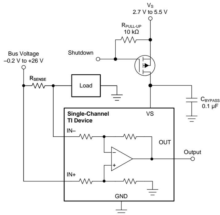
图 44. Basic Circuit to Shut Down the INx180
