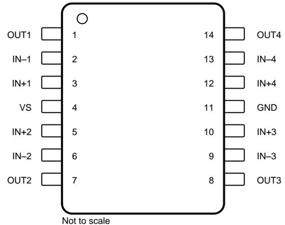
**Pin Functions: INA2180 (Dual Channel) and INA4180 (Quad Channel)**
