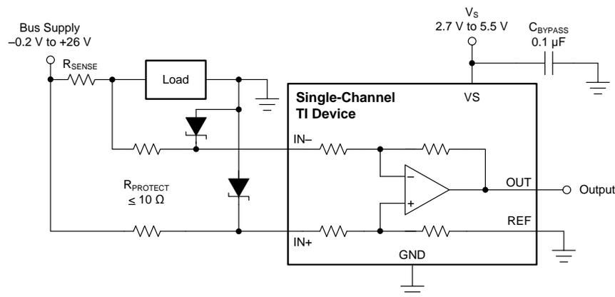
**图 55. Transient Protection Using Dual Zener Diodes**
