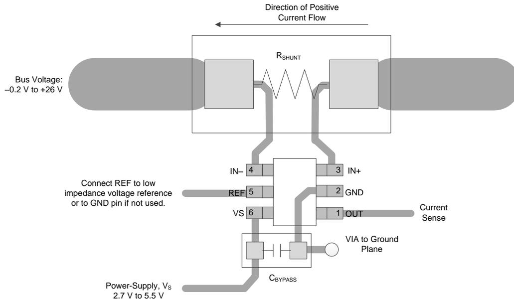
图 57. Single-Channel Recommended Layout
