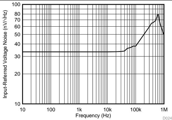
图 29. Input-Referred Voltage Noise vs Frequency (A3 Devices)
