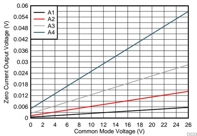
图 43. Zero-Current Output Voltage vs Common-Mode Voltage
