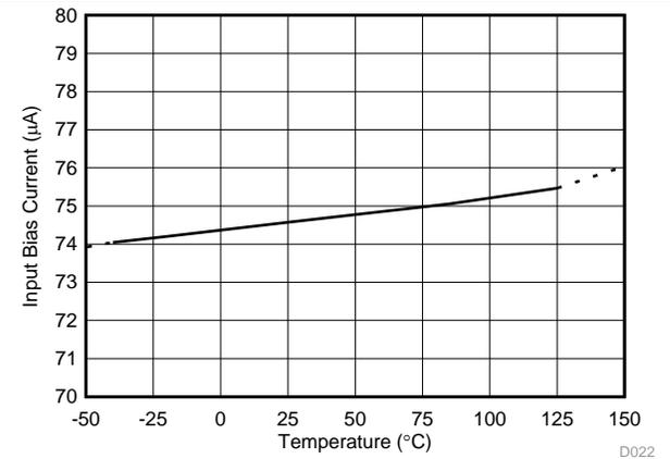
图 22. Input Bias Current vs Temperature
