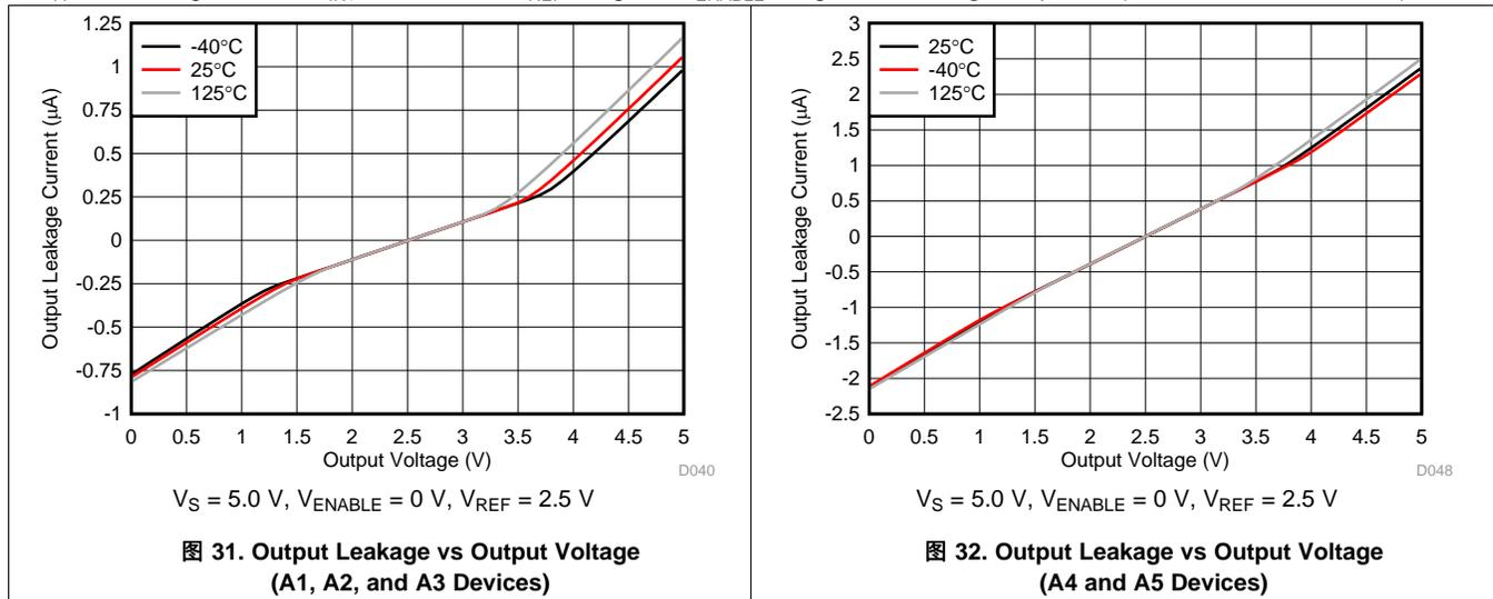
图 31. Output Leakage vs Output Voltage (A1, A2, and A3 Devices)
