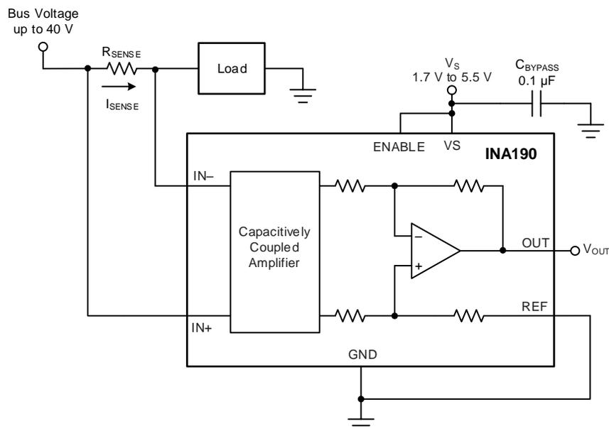
**图 35. Typical Unidirectional Application**
