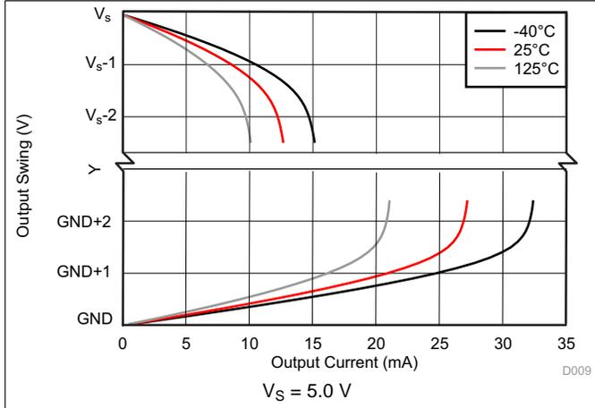
图 13. Output Voltage Swing vs Output Current
