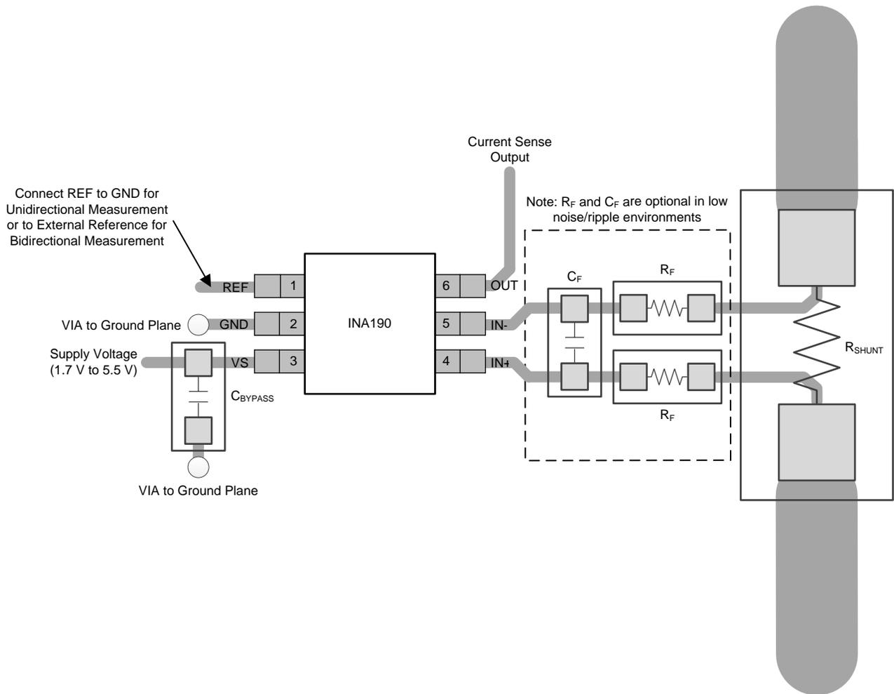
图 47. Recommended Layout for SC70 (DCK) Package
