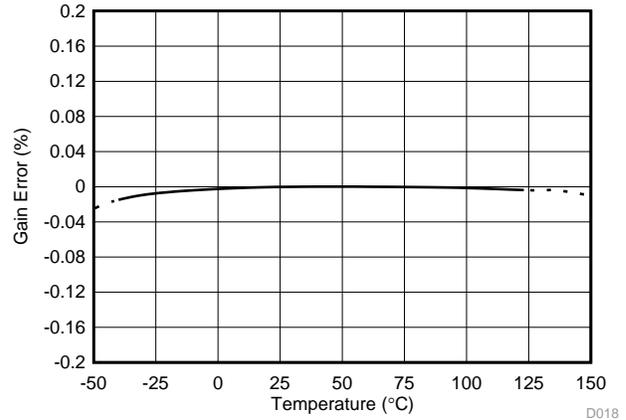
图 8. Gain Error vs Temperature
