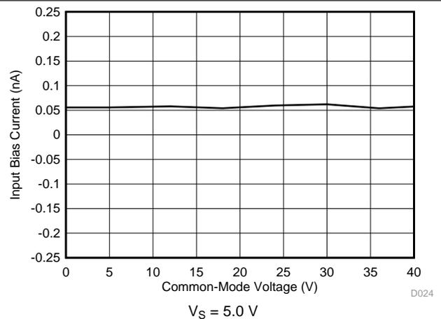
图 14. Input Bias Current vs Common-Mode Voltage
