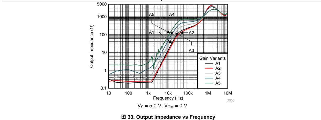
图 33. Output Impedance vs Frequency
