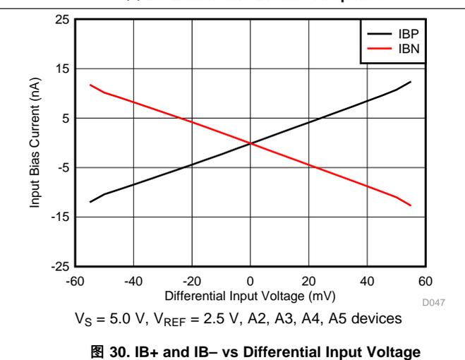
图 30.  $IB+$  and  $IB-$  vs Differential Input Voltage
