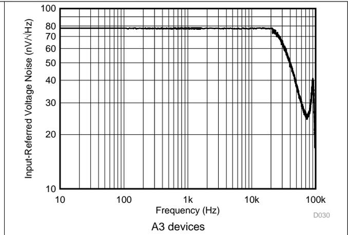
图 20. Input-Referred Voltage Noise vs Frequency
