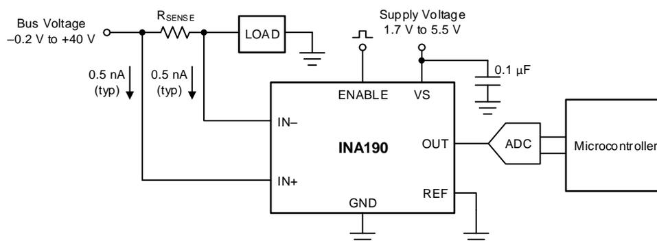
NOTE: To help eliminate ground offset errors between the device and the analog-to-digital converter (ADC), connect the REF pin to the ADC reference input. When driving SAR ADCs, filter or buffer the output of the INA190 before connecting directly to the ADC.
