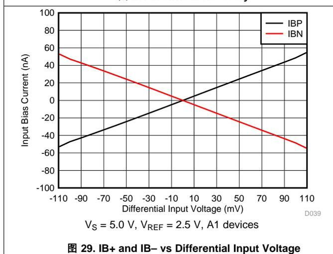
图 29.  $IB+$  and  $IB-$  vs Differential Input Voltage
