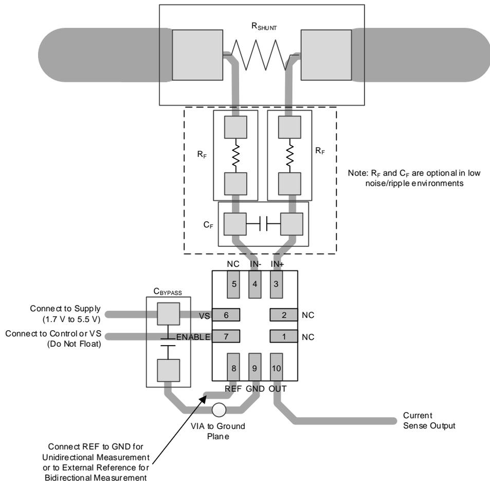
图 46. Recommended Layout for UQFN (RSW) Package
