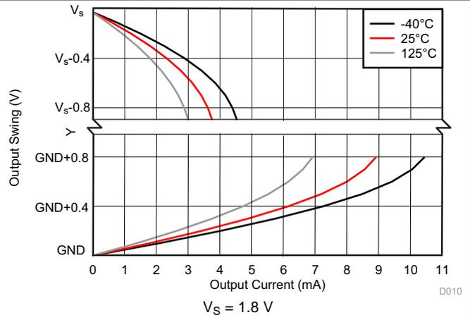
图 12. Output Voltage Swing vs Output Current
