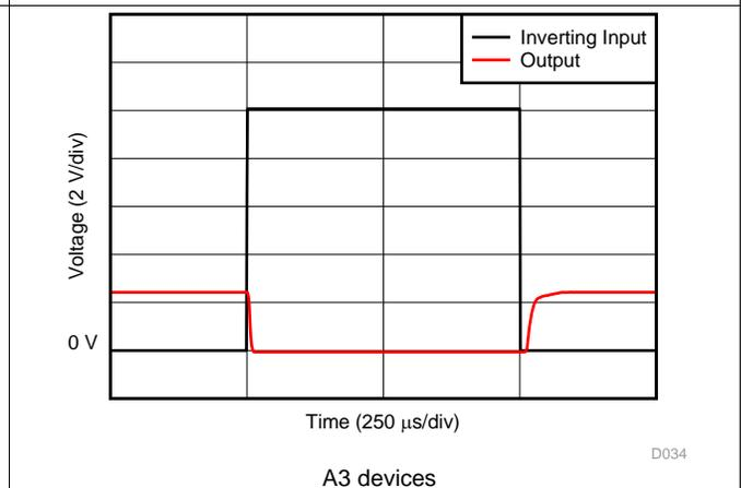
图 24. Inverting Differential Input Overload
