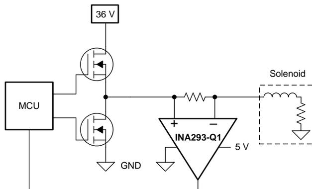
Figure 3. Current Sensing in a Solenoid Application
