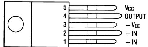
\*The tab is internally connected to pin 3 (-VEE)
