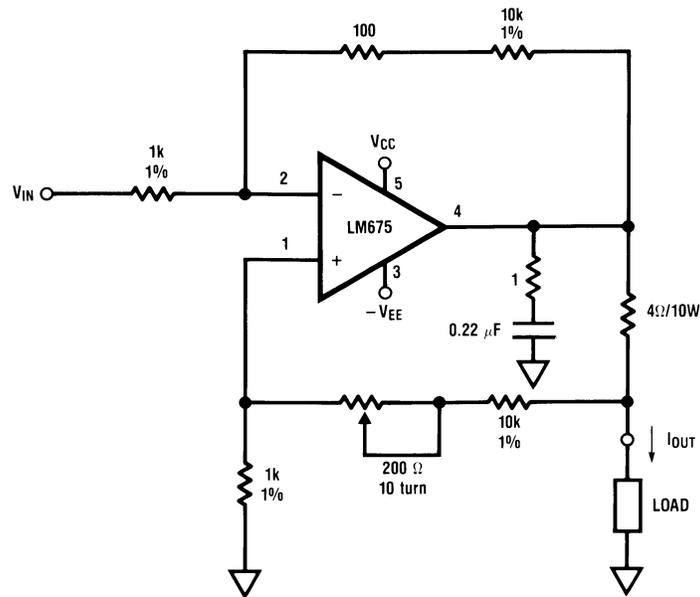
$I_{OUT} = V_{IN} \times 2.5 \text{ amps/volt}$
