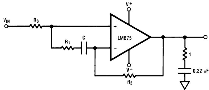
$$R_1 C \geq \frac{1}{2\pi 500 \text{ kHz}}$$
