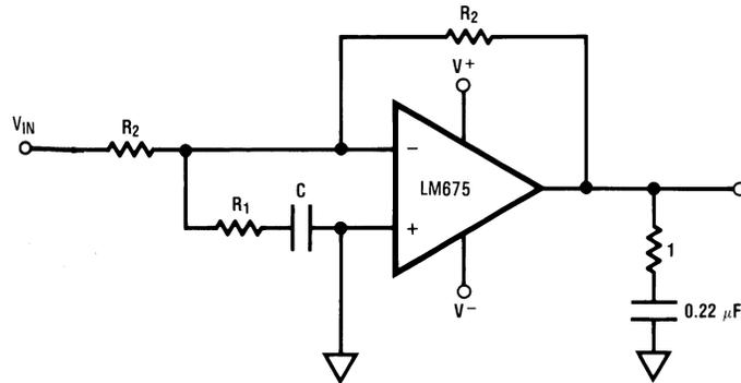
$$R_1 C \geq \frac{1}{2\pi 500 \text{ kHz}}$$
