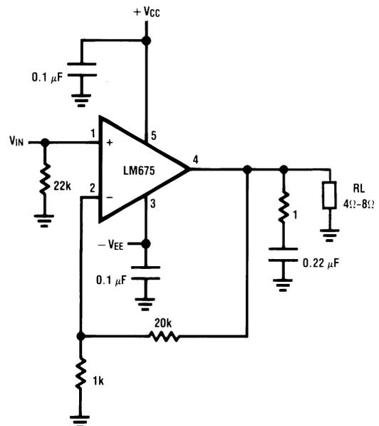
**Figure 2. Non-Inverting Amplifier**
