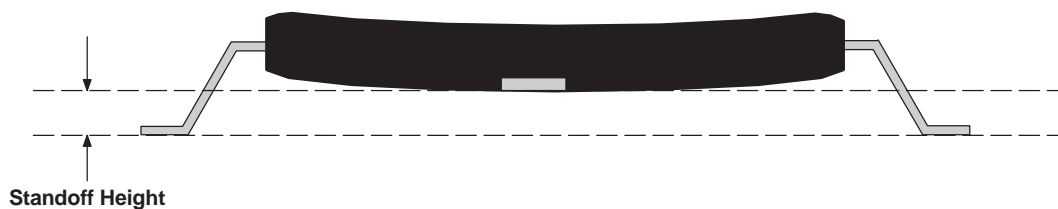
Figure 7-3. Standoff Height Measurement on 176-pin PTP Package
