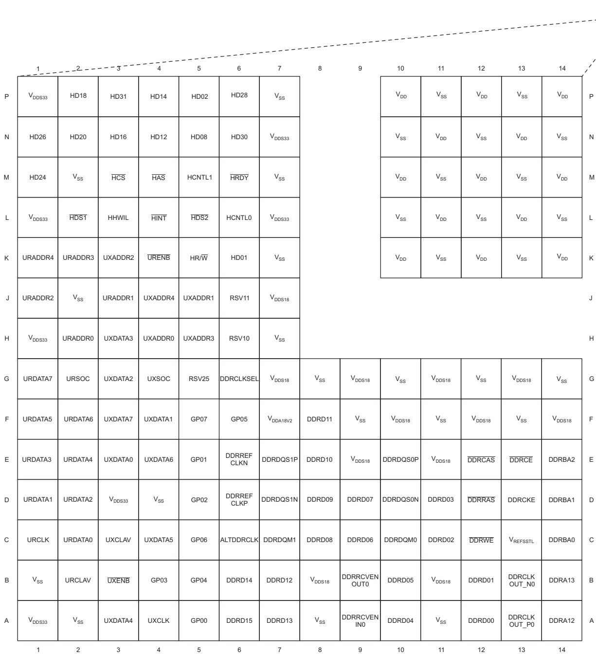
Figure 3-5. TCI648F Pin Map (Bottom View) [Quadrant D]
