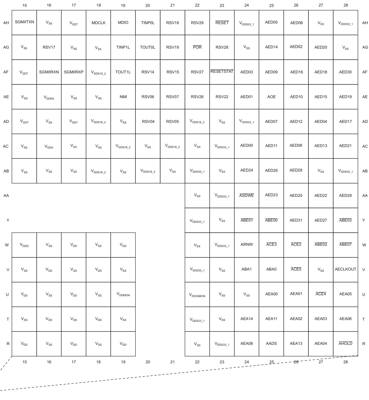
Figure 3-3. TCI648F Pin Map (Bottom View) [Quadrant B]
