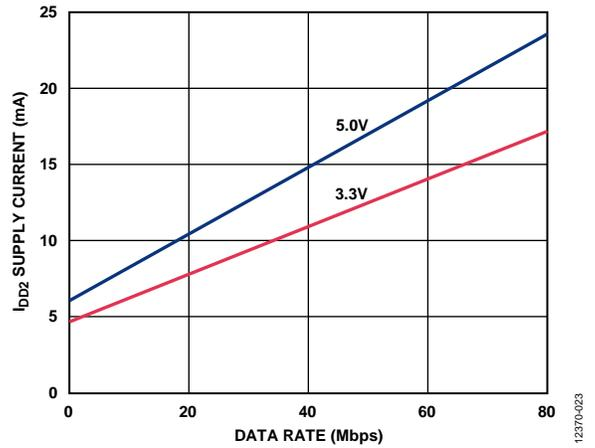
Figure 12. Typical I<sub>DD2</sub> Supply Current vs. Data Rate for 5.0 V and 3.3 V Operation
