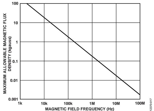
Figure 17. Maximum Allowable External Magnetic Flux Density
