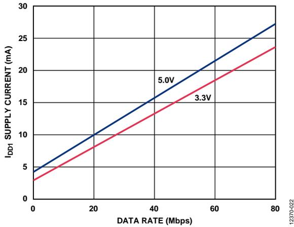
Figure 9. Typical I<sub>DD1</sub> Supply Current vs. Data Rate for 5.0 V and 3.3 V Operation
