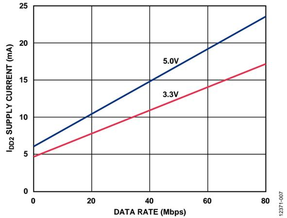
Figure 7. Typical I<sub>DD2</sub> Supply Current vs. Data Rate for 5.0V and 3.3V Operation
