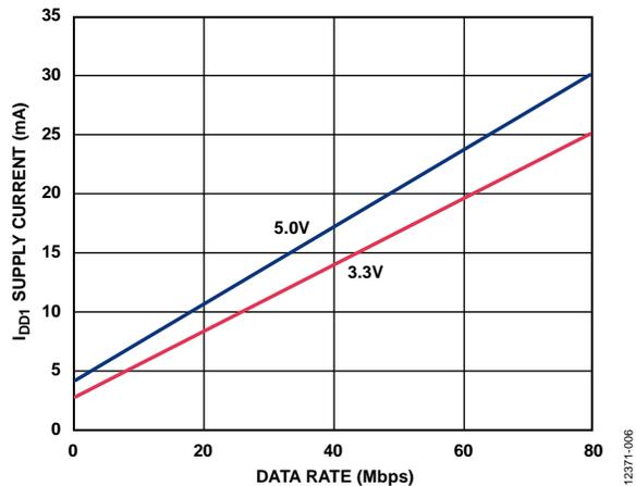
Figure 6. Typical I<sub>DD1</sub> Supply Current vs. Data Rate for 5.0V and 3.3V Operation
