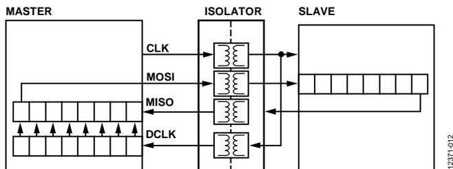
Figure 12. High Speed SPI Using Isolation Channel Delay
