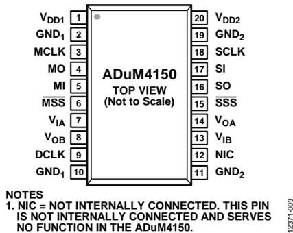
Figure 3. Pin Configuration
