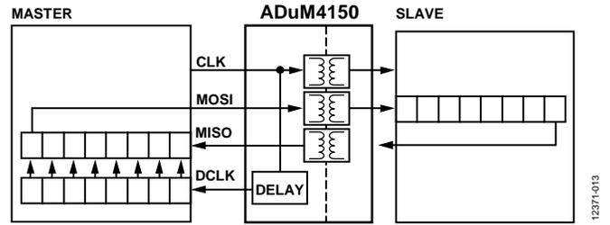
Figure 13. High Speed SPI Using Precision Clock Delay
