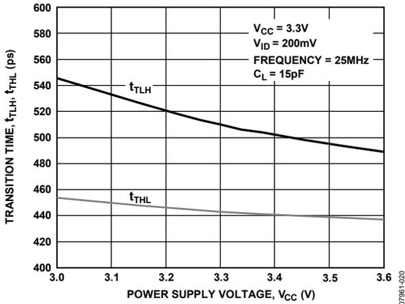
Figure 17. Transition Time vs. Power Supply Voltage
