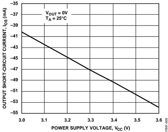
Figure 7. Output Short-Circuit Current vs. Power Supply Voltage
