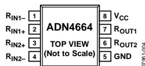
Figure 4. Pin Configuration
