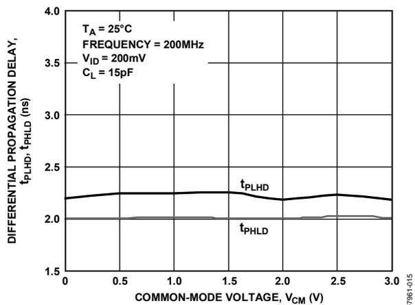
Figure 12. Differential Propagation Delay vs. Common-Mode Voltage
