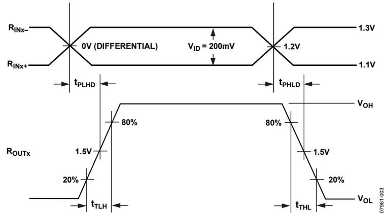
Figure 3. Receiver Propagation Delay and Transition Time Waveforms
