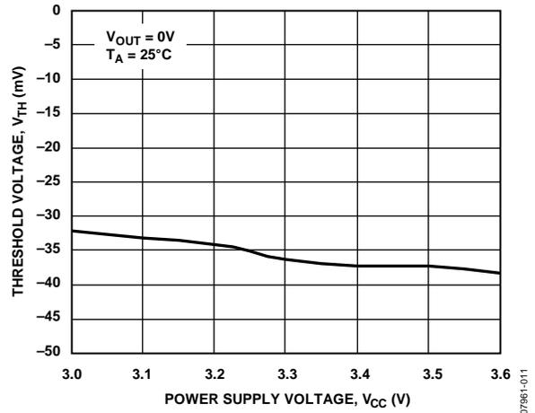
Figure 8. Threshold Voltage vs. Power Supply Voltage
