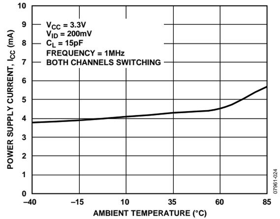
Figure 10. Power Supply Current vs. Ambient Temperature
