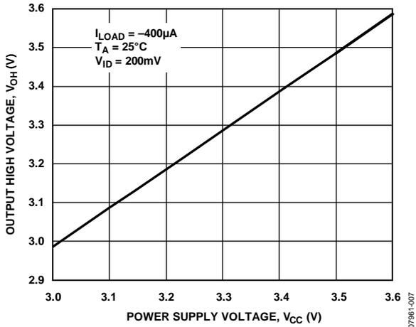
Figure 5. Output High Voltage vs. Power Supply Voltage
