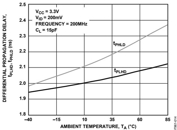
Figure 11. Differential Propagation Delay vs. Ambient Temperature
