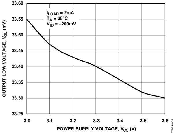
Figure 6. Output Low Voltage vs. Power Supply Voltage
