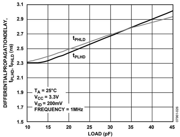
Figure 19. Differential Propagation Delay vs. Load at 1 MHz
