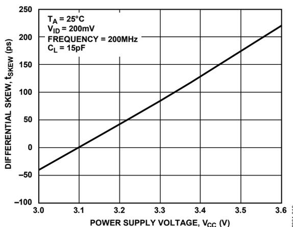
Figure 15. Differential Skew vs. Power Supply Voltage
