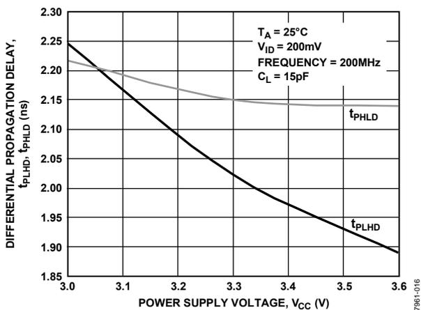
Figure 13. Differential Propagation Delay vs. Power Supply Voltage
