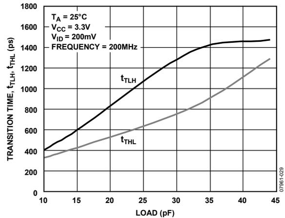
Figure 22. Transition Time vs. Load at 200 MHz
