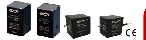
EOT's Amplified Photodetectors contain PIN photodiodes that utilize the photovoltaic effect to convert optical power into an electrical current and a fixed gain transimpedance amplifier allowing measurement of <1 mW input powers.
