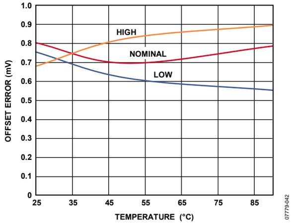
Figure 27. MV Offset Error vs. Temperature, MEASOUT Gain = 1
