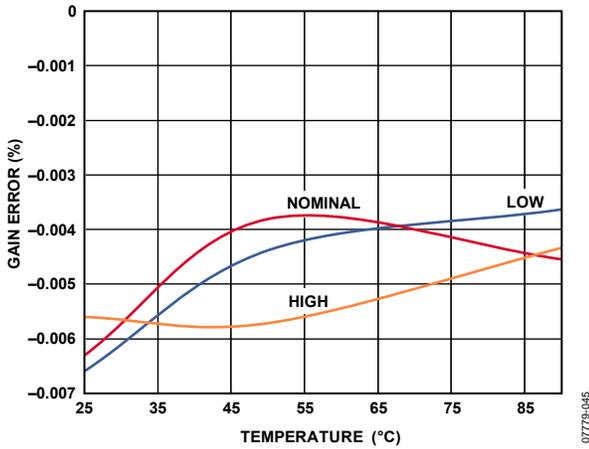
Figure 26. MV Gain Error vs. Temperature, MEASOUT Gain = 1
