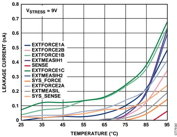
Figure 21. Leakage Current vs. Temperature,  $V_{STRESS} = 9V$
