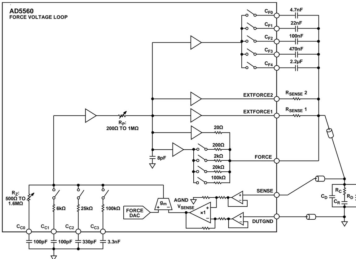
Figure 57. Block Diagram of a Force Amplifier Loop
