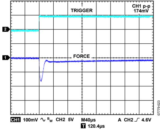
Figure 38. Safe Mode 10% to 90%, EXTFORCE2 Range, 10 µF Load
