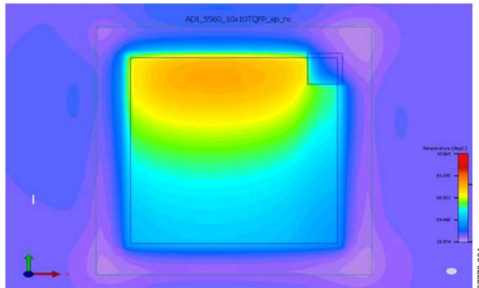
Figure 62. Temperature Contour Map for 64-Lead TQFP\_EP
