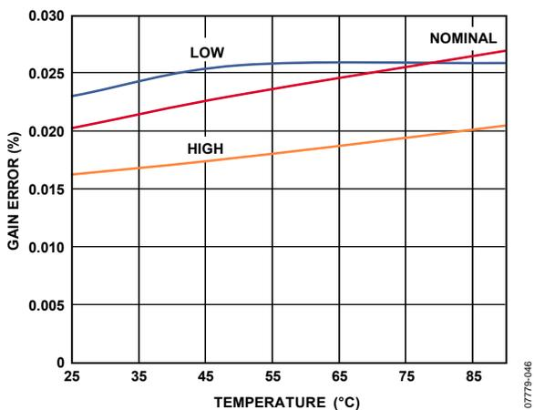
Figure 28. MV Gain Error vs. Temperature, MEASOUT Gain = 0.2
