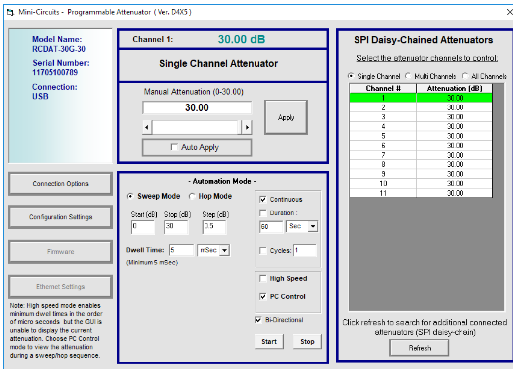
RCDAT GUI main screen (USB control) with 11 units connected in series
