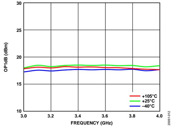
Figure 15. OP1dB vs. Frequency at Various Temperatures
