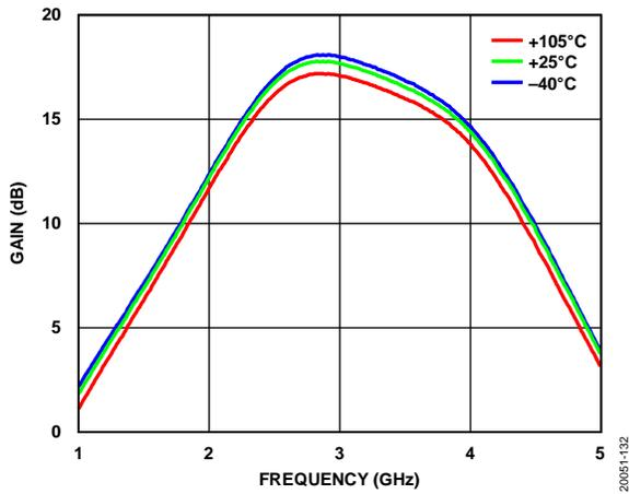
Figure 35. Gain vs. Frequency at Various Temperatures
