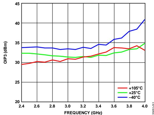
Figure 13. OIP3 vs. Frequency, 8 dBm Output Tone Power
