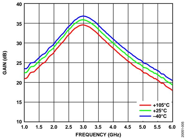
Figure 8. Gain vs. Frequency at Various Temperatures
