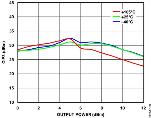
Figure 33. OIP3 vs. Output Power, 2.6 GHz
