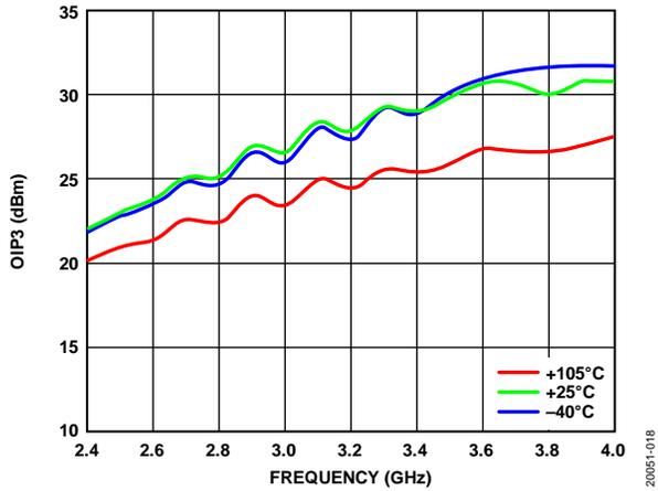
Figure 21. OIP3 vs. Frequency, -10 dBm Output Tone Power
