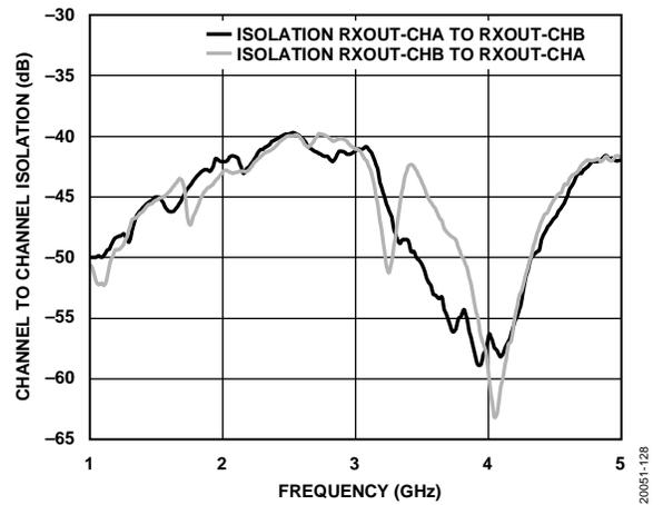
Figure 31. Channel to Channel Isolation vs. Frequency
