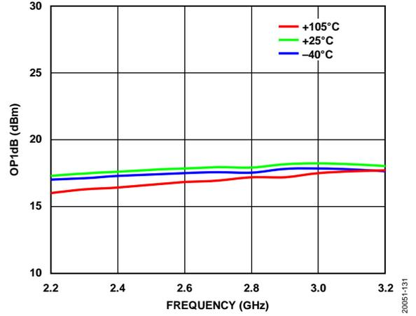
Figure 34. OP1dB vs. Frequency at Various Temperatures
