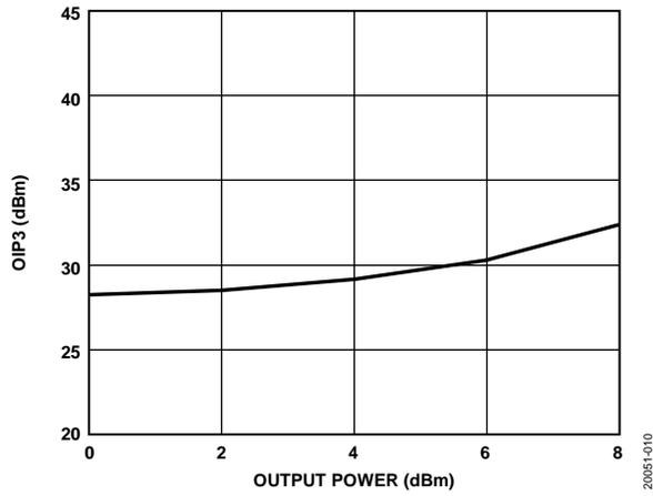
Figure 14. OIP3 vs. Output Power, 3.6 GHz
