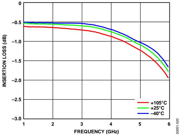
Figure 23. Insertion Loss vs. Frequency at Various Temperatures
