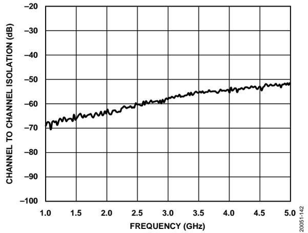
Figure 45. Channel to Channel Isolation vs. Frequency
