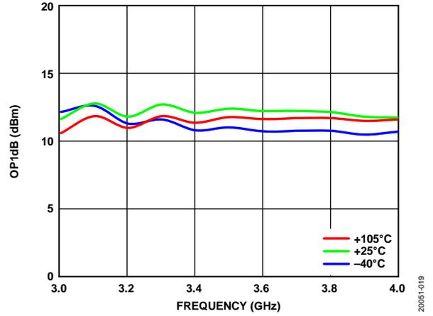
Figure 22. OP1dB vs. Frequency at Various Temperatures
