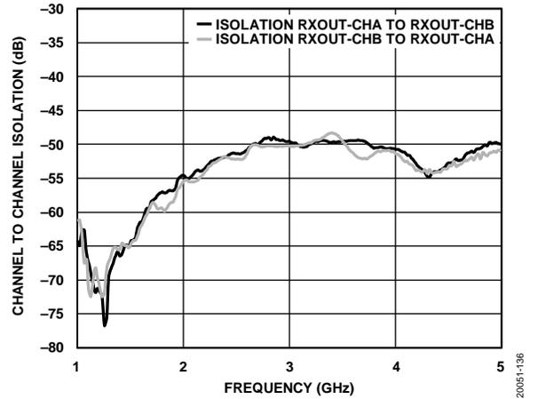
Figure 39. Channel to Channel Isolation vs. Frequency
