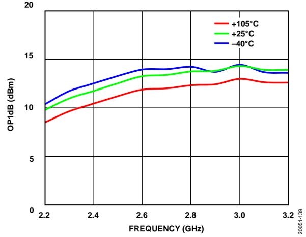
Figure 42. OP1dB vs. Frequency at Various Temperatures
