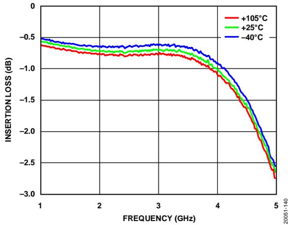
Figure 43. Insertion Loss vs. Frequency at Various Temperatures
