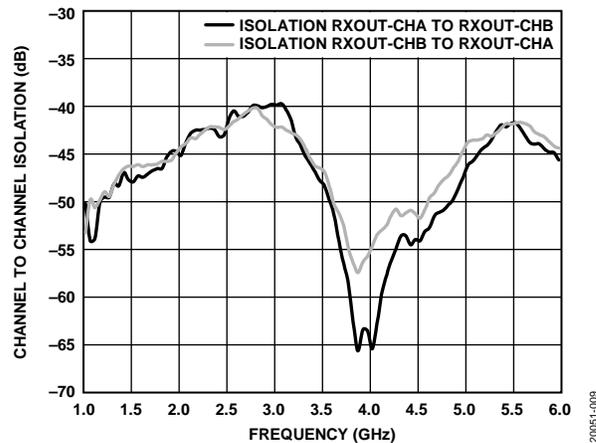
Figure 12. Channel to Channel Isolation vs. Frequency
