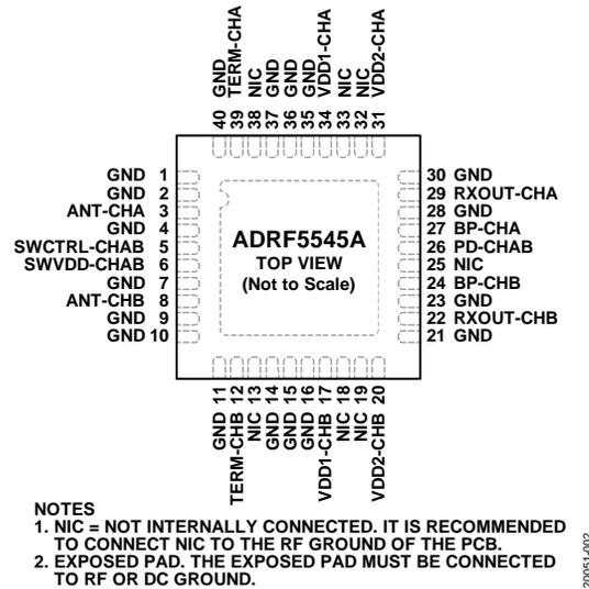
Figure 2. Pin Configuration
