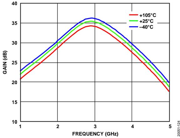
Figure 27. Gain vs. Frequency at Various Temperatures
