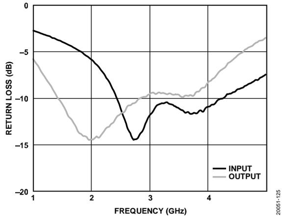
Figure 28. Return Loss vs. Frequency
