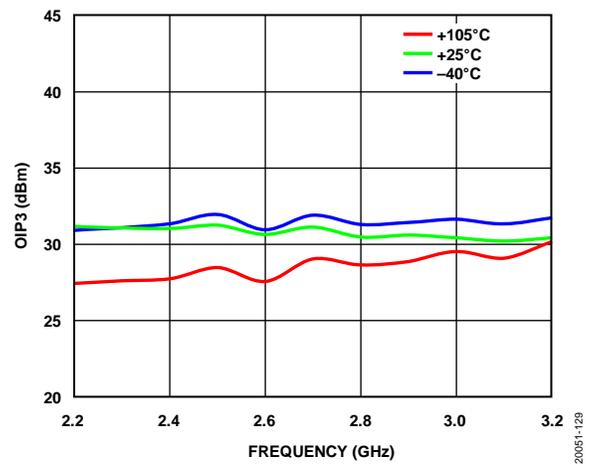
Figure 32. OIP3 vs. Frequency, 8 dBm Output Tone Power
