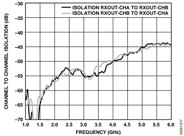
Figure 19. Channel to Channel Isolation vs. Frequency
