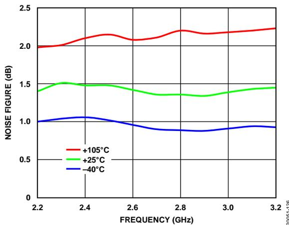
Figure 29. Noise Figure vs. Frequency at Various Temperatures
