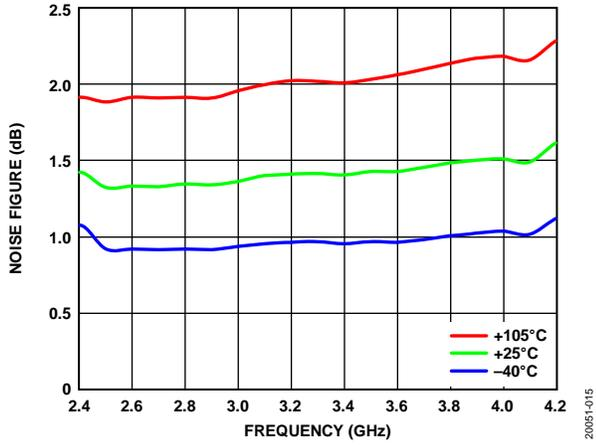
Figure 20. Noise Figure vs. Frequency at Various Temperatures
