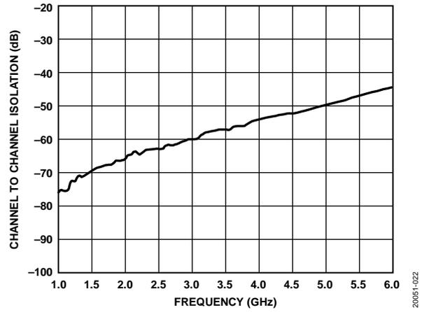
Figure 25. Channel to Channel Isolation vs. Frequency
