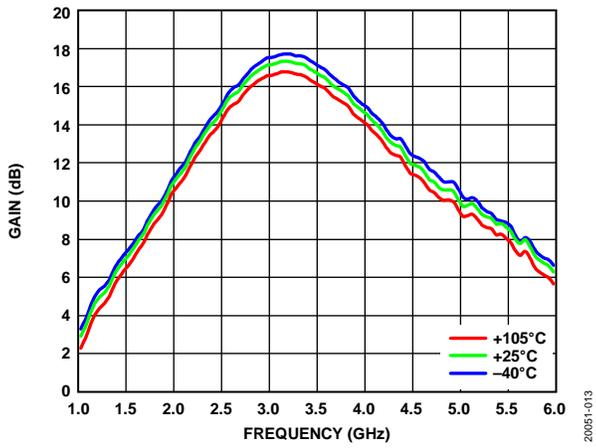
Figure 16. Gain vs. Frequency at Various Temperatures
