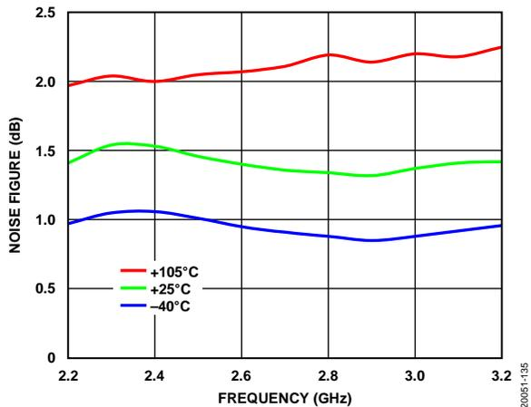
Figure 37. Noise Figure vs. Frequency at Various Temperatures
