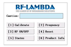
To enter this function selection page, press "Menu" on front panel keypad while the instrument is showing the status page.
