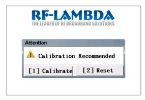
Calibration is may be recommended "[1] Calibrate" to execute instrument self calibration process.
