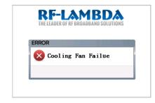
The front panel LCD screen will display the error code or error message when instrument self protection is triggered. Front panel alarm indicator will light up.
