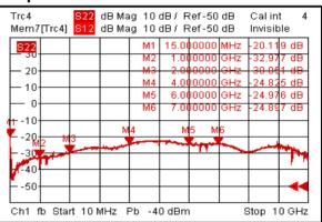
Note: Input/output return loss measurements include attenuators to protect equipment
