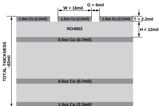
Figure 41. Probe Matrix Board Stackup
